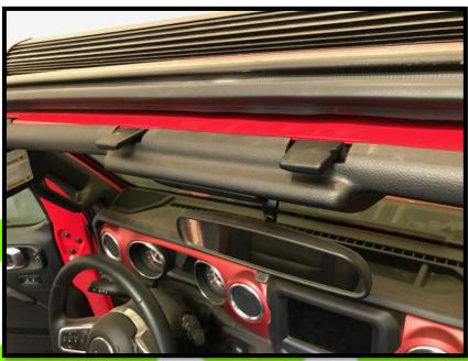
For the rear 2 brackets there are 3 bolts that need to be removed that will allow you to access the bolt holes for the rear brackets (see below). Again there is a left and a right. They should be configured so that the holes are toward the outside of the Jeep (see below)
