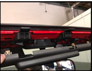
The front brackets will look like the photo below and will be marked with the letter L and R. The L bracket goes towards the driver's side and the R bracket goes to the passenger side. There will be threaded holes where these will install. The hardware that was sent will contain 4 bolts to connect these front 2 brackets. There may be paint in the holes that makes the installation of the bolts more difficult.
