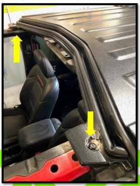
4. Make sure that the top is aligned evenly on the Jeep. Comparing the distances at the seal with back of the rear door jam shown in figure 4. Make sure that the seal lines up with the top. Tighten the 6 bolts on the tub in a star pattern (Fig 5) while an assistant ensures that the top remains in position, you may need to push on the top like in figure 4 to get it into position.
